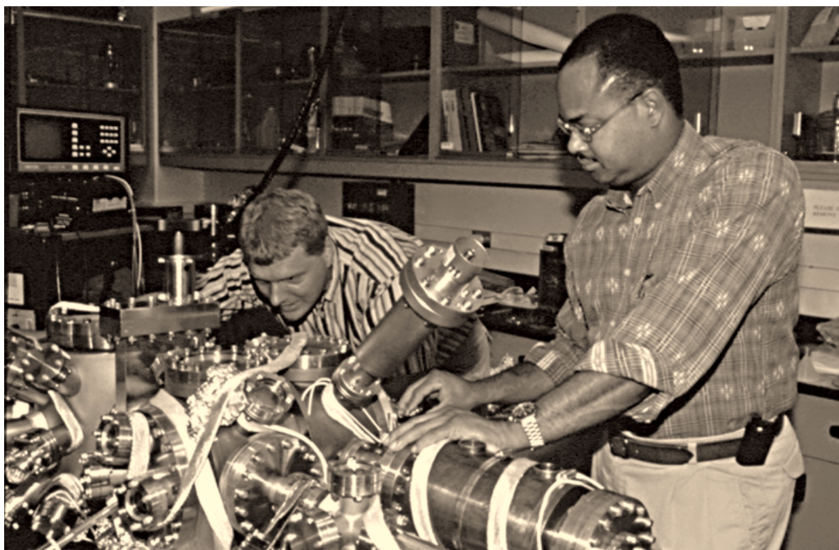
Science and Engineering of Materials student John Edwards, right, and research scientist Peter Fuchs use a scanning tunneling microscope to study a new phase on a silicon surface.
