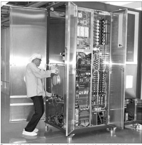
The vertical diffusion furnace was the first piece of equipment to be delivered and installed in the Teaching Factory, located in the Technology Center at ASU East. Tim Trumble photo
