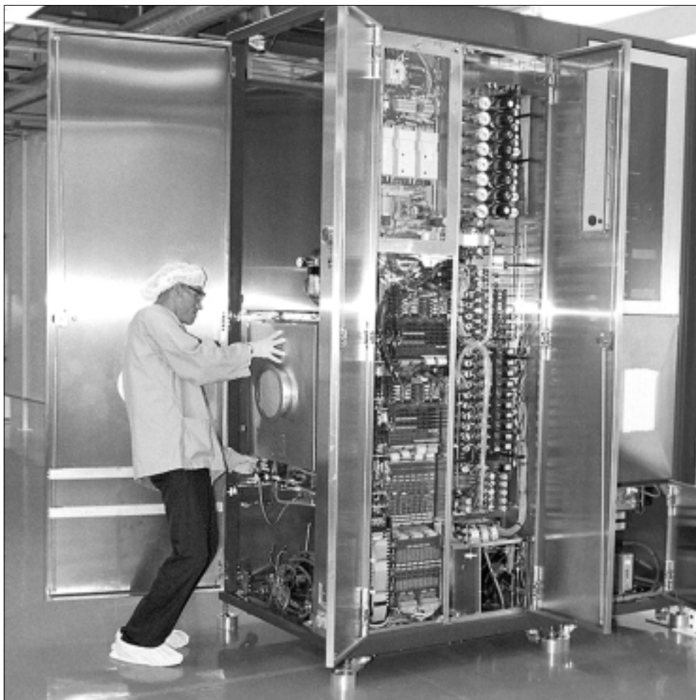
The vertical diffusion furnace was the first piece of equipment to be delivered and installed in the Teaching Factory, located in the Technology Center at ASU East.
