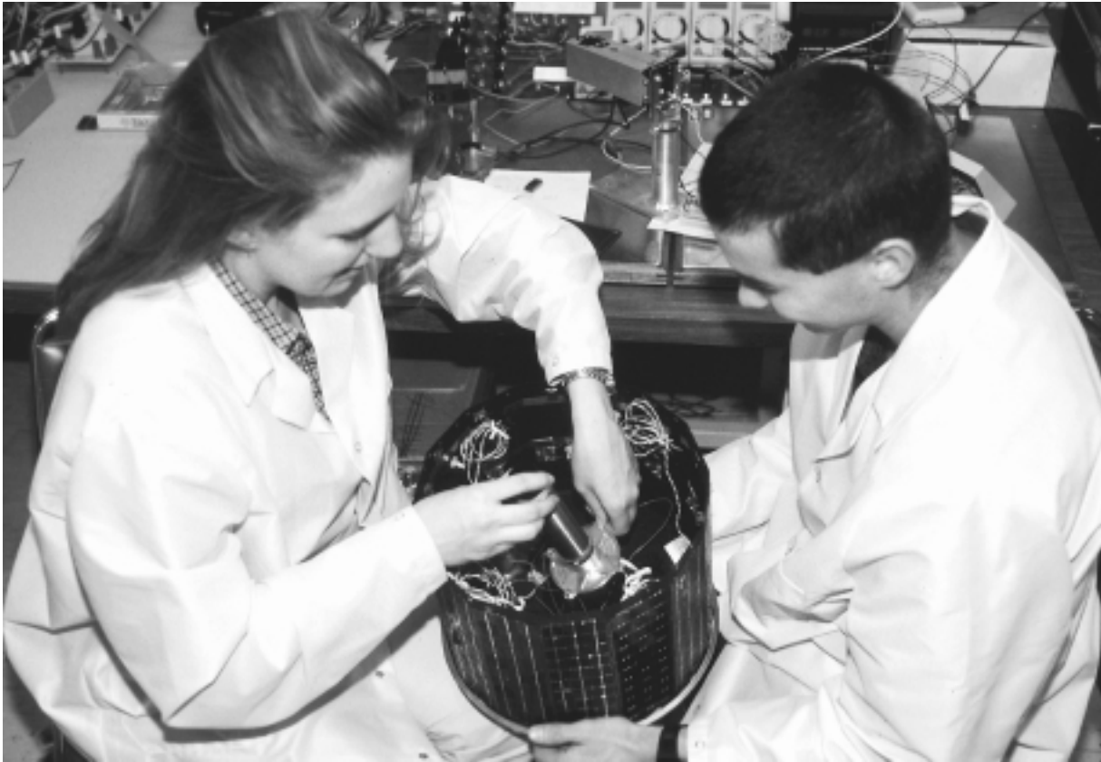
Engineering students assemble ASUSat1. The satellite, designed to map earth features, is a student-initiated project that has involved more than 400 students over the past six years.
