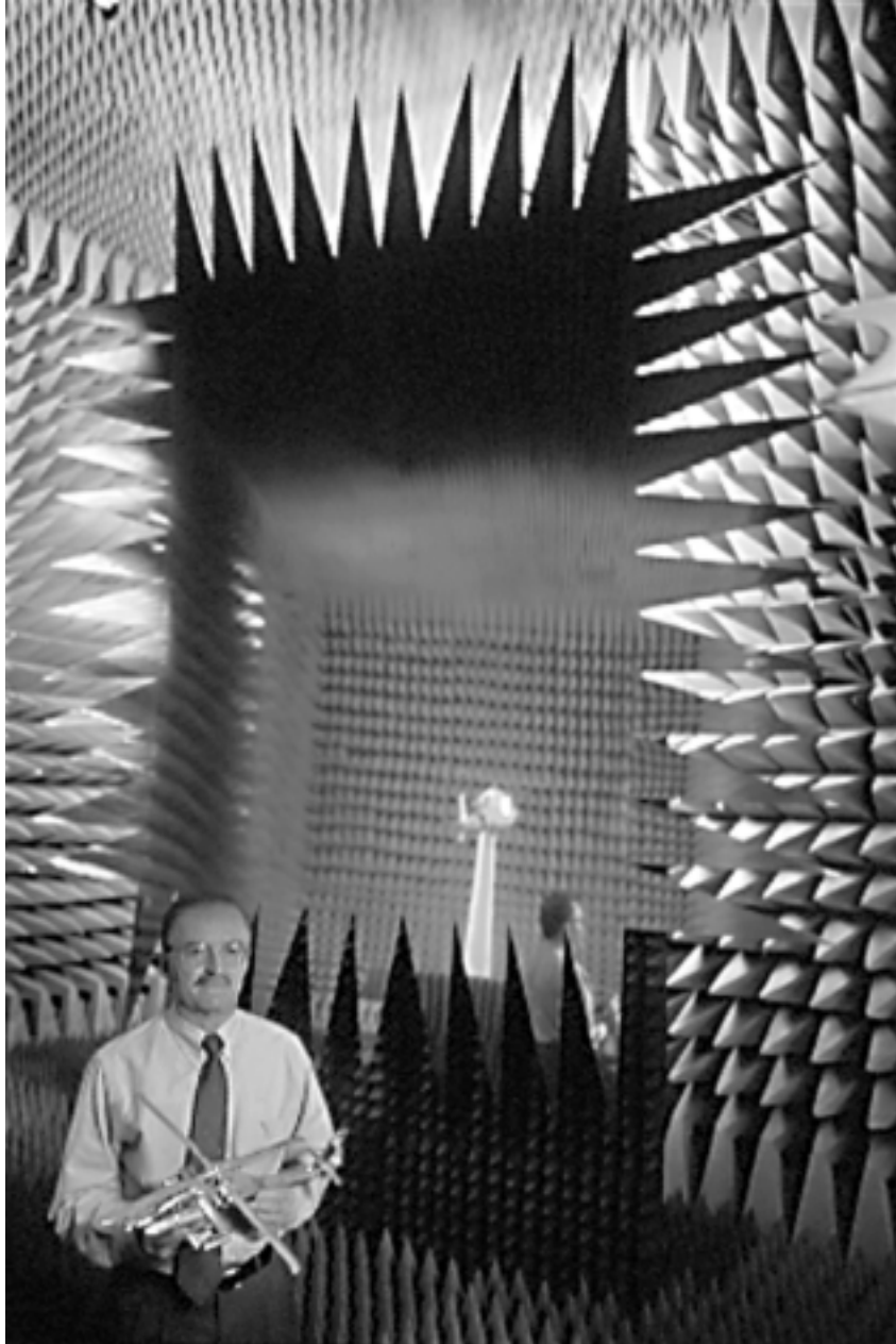
Regents' Professor of Electrical Engineering Constantine Balanis stands in the Electromagnetic Anechoic Chamber. The chamber provides a controlled environment for radar cross-section and antenna radiation pattern measurements.
