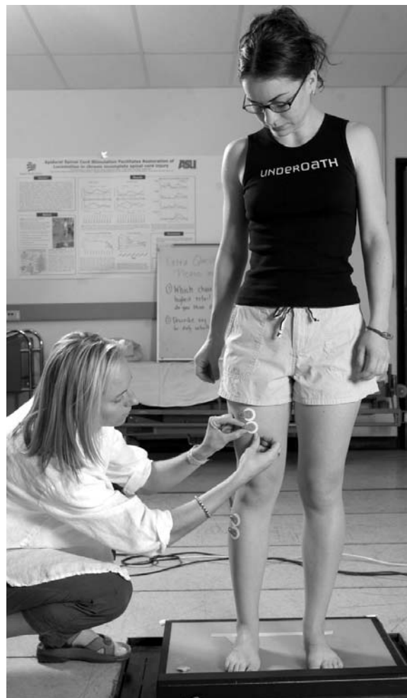
Kristine Csavina, a doctoral student in bioengineering, attaches electrodes to a student as part of an experiment that evaluates balance changes in the aging process. Tim Trumble photo
