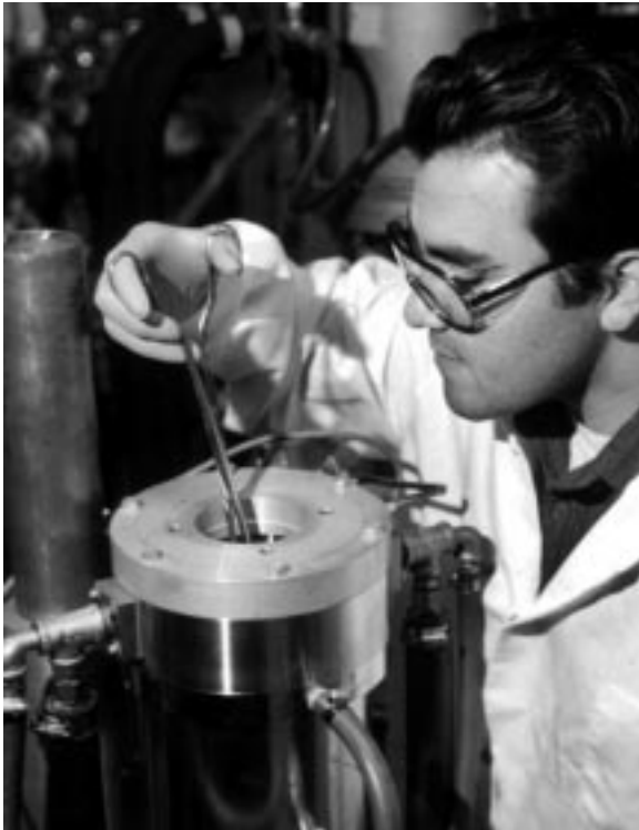
A student in the materials facility prepares to heat treat an aluminum alloy for aerospace research with a high-temperature refractory-metal furnace.
