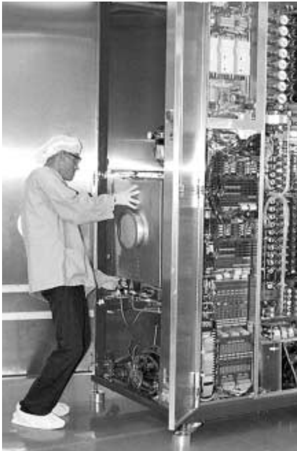
The vertical diffusion furnace was the first piece of equipment to be delivered and installed in the Teaching Factory, located in the Technology Center at ASU East.
